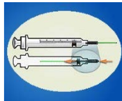
Figure 4 Syringe with a Retractable Needle
